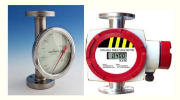
**"INSTONNIC"** make Metal Tube Rota meter is a variable area flow meter MTR series is suitable for gas and liquid flow measurement even under high pressure and high temperature. Standard flow tube is in SS 316 and for corrosive applications the metal tube, orifice and float can be lined with PTFE. Metal Tube Rotameter comes with optional limit switches and 4-20ma output.
